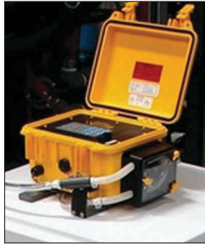
"Water Clear" lid allows easy inspection of rollers and tubing.
