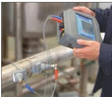
DXN Flowmeter uses non-invasive ultrasonic technology and straps to outside of pipe
