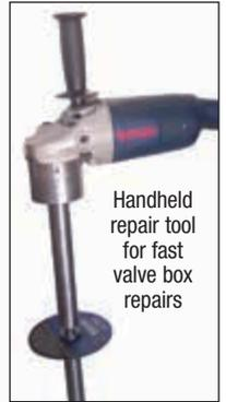
Handheld repair tool for fast valve box repairs
