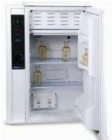
This space saving BOD incubator can sit on the floor or on top of your bench. Forced air circulation and microprocessor-based PID control ensure stable and uniform temperature throughout the chamber. LED displays both setpoint and chamber temperature. Additional features include over-temperature protection and an interior electrical outlet that can handle a 1A load.
